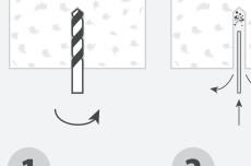
Drill a  $\emptyset$  6 mm hole of the required length.
